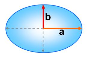
Flattening is the ratio of the difference between the Semi-Major Axis, and the Semi-Minor Axis.
