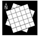
The ADM<sup>SAR</sup> product is an orbit merge, i.e. a combination of SAR images from ascending and descending right looking orbits is used for image analysis. This achieves a reduction of the impact of the typical SAR effects of shadow and layover, which are usually visible and may obscure parts of the area under investigation.
