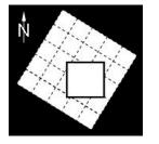
The Oriented Image is a subset of an orthorectified or geocoded image scene, a mosaic or an ascending / descending merge. The subset region is defined by the customer via an Area of Interest polygon or corner coordinates of the desired region. The product can either be characterised by the user defined Area of Interest or by a map sheet orientation according to relevant mapping standards or customer defined extensions.
