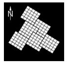
In order to cover a geographical area larger than a standard scene, neighbouring geocoded or orthorectified images are combined into one image in a seamless way. Supported input products are ORI<sup>SAR</sup>, EEC or GEC depending on the customer's localisation accuracy requirements.
