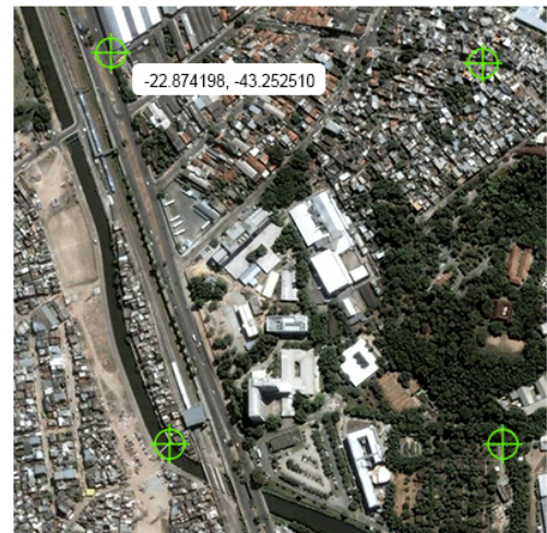
Assign world coordinates to the control points (WX and WY). These can be assigned manually or by using an online map service to do it interactively.
