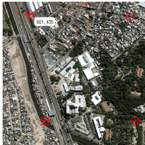
Add control points to an unreferenced image that are easy to identify when adding world coordinates. Control points are assigned pixel coordinates (PX and PY).
